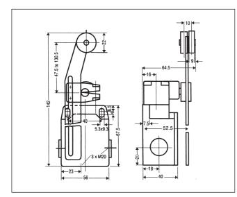
Limit Switch with Roller Crank 3SE3 100-0U
