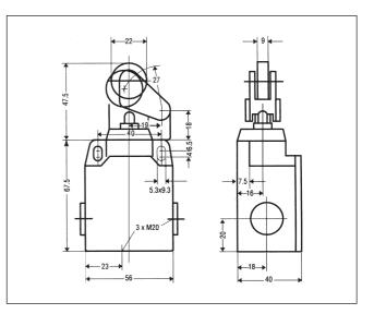
Limit Switch with Roller Lever 3SE3 100-0E
