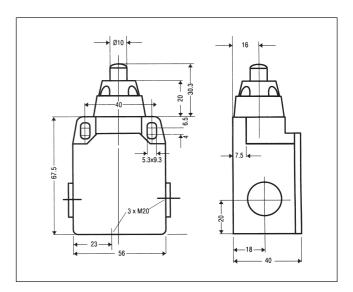
Limit Switch with Overtravel plunger 3SE3 100-0C
