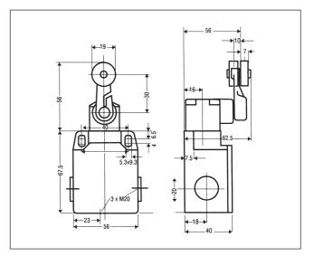
Limit Switch with Roller Crank 3SE3 100-0G
