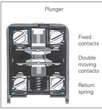
Fig. 4 Slow-action switch with 1 NO + 1NC
