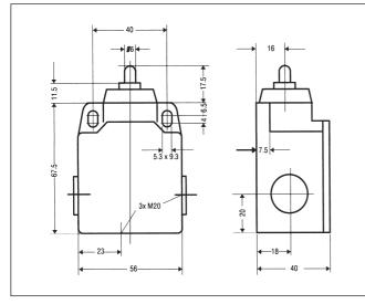
Limit Switch with Plunger 3SE3 100-0B
