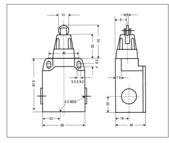
Limit Switch with Roller Plunger 3SE3 100-0D
