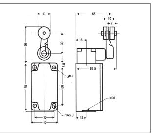
Limit Switch with Crank Lever 3SE3 120-0G
